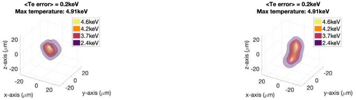
FIGURE B.10. 3D T_e measurement using 2 LOS at (30^\circ, 30^\circ) (left) and (210^\circ, 30^\circ) (right)
