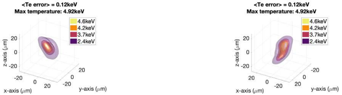
FIGURE B.11. 3D T_e measurement using 3 LOS at (30^\circ, 30^\circ) (left) and (210^\circ, 30^\circ) (right)
