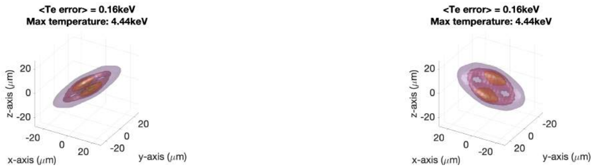
FIGURE B.23. 3D T_e measurement using 3 LOS at (30^\circ, 30^\circ) (left) and (210^\circ, 30^\circ) (right)
