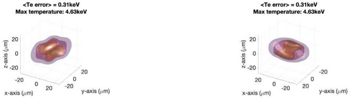
FIGURE B.22. 3D T_e measurement using 2 LOS at (30^\circ, 30^\circ) (left) and (210^\circ, 30^\circ) (right)
