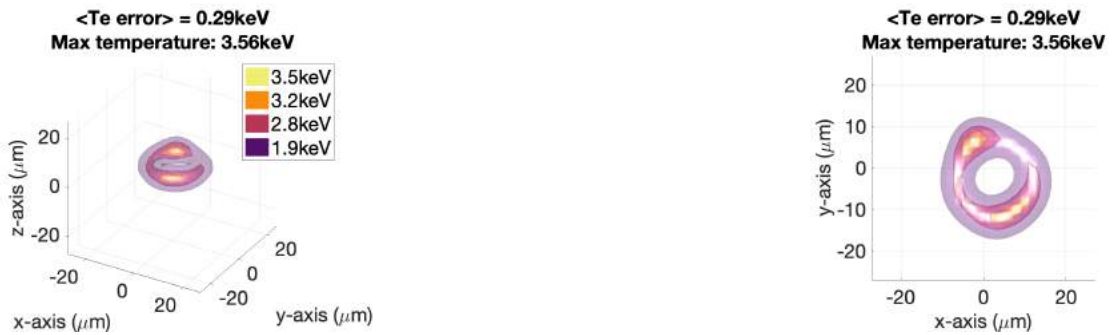
FIGURE B.18. 3D T_e measurement using 2 LOS at (30^\circ, 30^\circ) (left) and (0^\circ, 0^\circ) (right)
