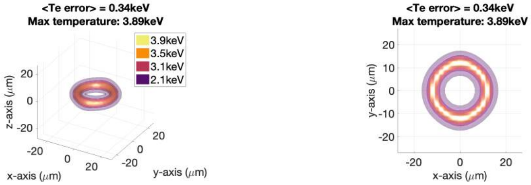
FIGURE B.14. 3D T_e measurement using 2 LOS at (30^\circ, 30^\circ) (left) and (0^\circ, 0^\circ) (right)
