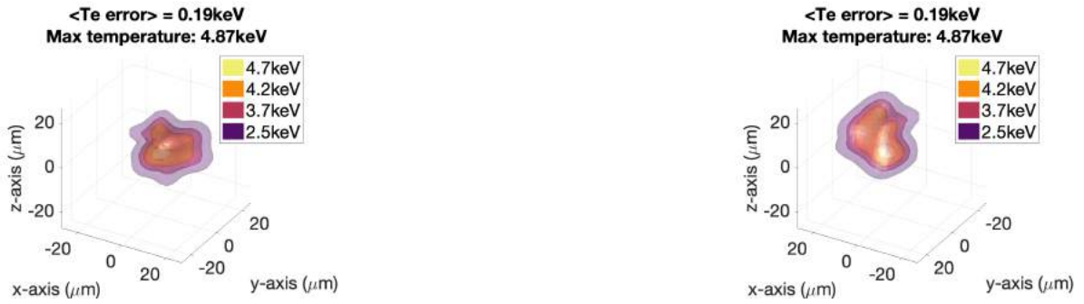
FIGURE B.2. 3D T_e measurement using 2 LOS at (30^\circ, 30^\circ) (left) and (210^\circ, 30^\circ) (right)
