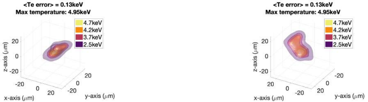
FIGURE B.3. 3D T_e measurement using 3 LOS at (30^\circ, 30^\circ) (left) and (210^\circ, 30^\circ) (right)
